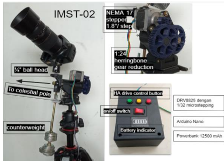
Figure 6. IMST-02 3d printed mini german equatorial mount
